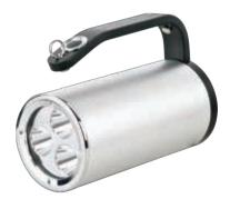
Ex marking: Ex d ib IIC T6 Gb Ex tD A21 IP68 T80°C
