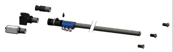
The objective lenses are separate optic systems which allow to change the direction of vision of the endoscope.
